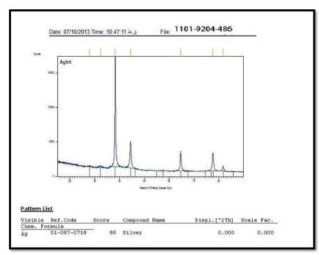
Fig.3. XRD pattern of silver nanoparticles obtained using Nasturtium Officinale R. Br. (NO).
