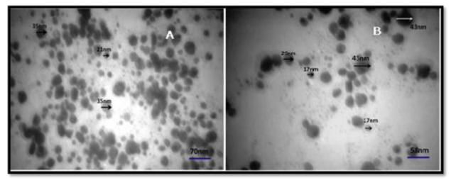
Fig.1. TEM images indicating the presence of spherical silver nanoparticles recorded at various magnifications (A and B).
