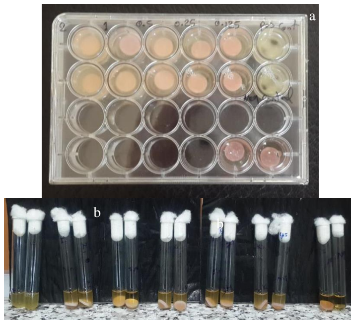
Figure 8. MIC of TiO 2 nanocomposites for S. mutans (a), and C. albicans (b)
