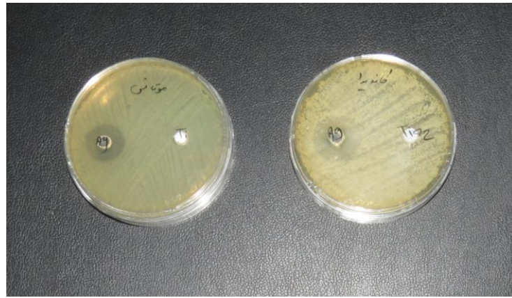
Figure 2. Growth inhibition zones caused by \text{TiO}_2 and AgNPs in S. mutans (left) and C. albicans (right) cultures
