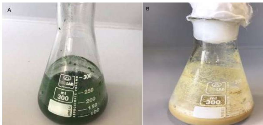
Figure 1. (A) suspension and chemicals, before and (B) after three stages of chemical treatment
